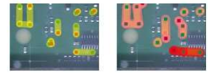
Seamlessly creates true-to-scale image of entire board Paint flux and solder paths to create and edit programs
